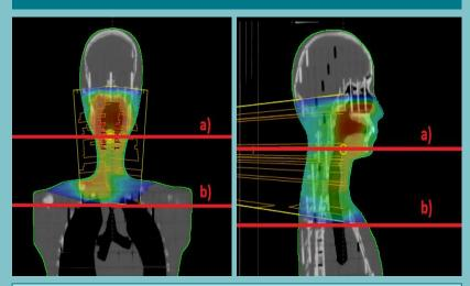
Doses were computed on the Eclipse TPS v.13.5 using the analytic anisotropic algorithm (AAA).
